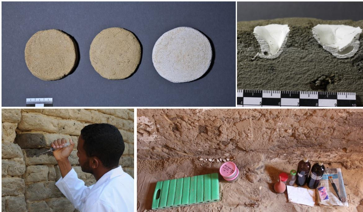
Fig. 2, 3: Empirical testing of conservation materials and recipes for the development i.e. of suitable conservation mortars and injection grouts.
