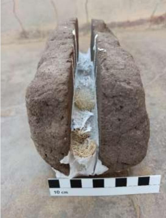
Grouting tests with Luffa pieces, filled between two mud bricks found in the desert
